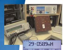
By incorporating this useful and easy to use option the work load of the calibrator can be increased to allow calibration of RLC (Resistance, Inductance and Capacitance) meters and bridges and also allows calibration of DMMs with inductance measurement ranges.
