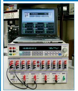
Automation of measurements with the addition of the 10-channel scanner greatly increases the versatility of the 8000 series. and allows a complete measurement system to be easily realised. The scanner together with the Pro raph software for PC makes an ideal combination for evaluating stability of measurements.
