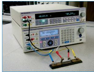
Dedicated shunt measurement function simplifies high current shunt measurement.
