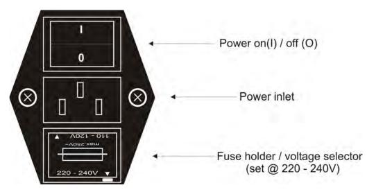
After connecting line power, the instrument can be switched on with the power switch on the rear of the instrument.
