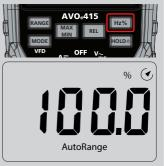
Press the Hz% button to return to current measurement
