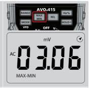
To exit MAX/MIN mode press and hold the MAX/MIN key for 2 seconds
