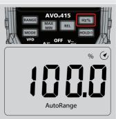
12. Press the Hz% button to return to the measurement
