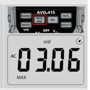
3. Press the MAX/MIN key again to activate the MIN recording mode.
