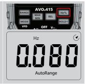
9. Press the Hz% button until "%" is indicate to read the % duty cycle in the display
