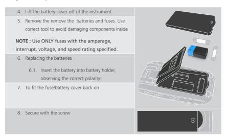
WARNING: To avoid electric shock, do not operate the meter until the battery cover is in place and fastened securely.
