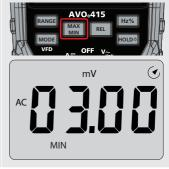
Press the MAX/MIN key again to activate the MAX/MIN recording mode.
