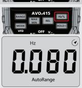
11. Press the Hz% button until "%" is indicate to read the % duty cycle in the display
