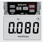
12. Press the Hz% button until "%" is indicate to read the % duty cycle in the display
